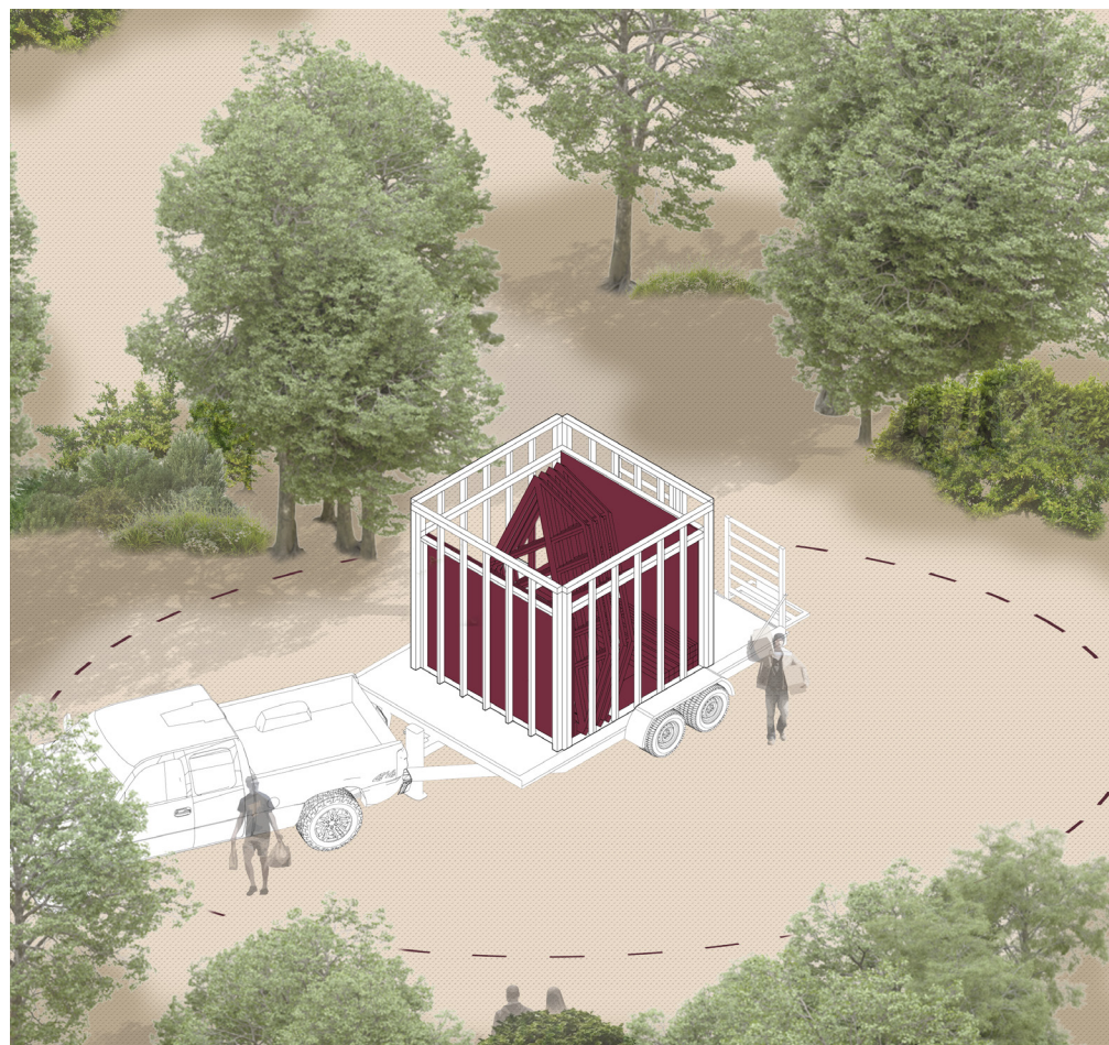
The movable gallery arrives prefabricated, fitting the dimensions of a standard trailer. All pieces of the gallery fit within the core frame of the gallery.
