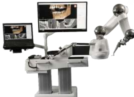
Figure 2: The First Dental Robot: Configuration of the Yomi dental robotic system (Parmar, 2017).
