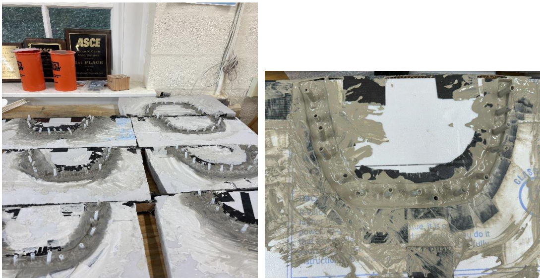
Figure 6: Concrete Placed in Molds
