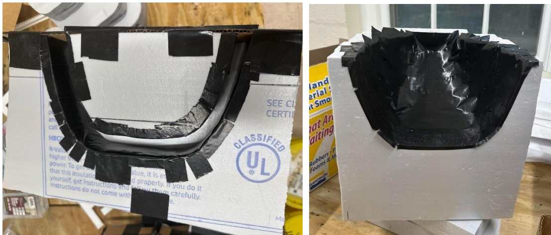
Figure 4: Injection and Female Molds
