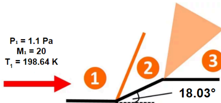
Figure 9: Oblique shock followed by expansion fan
