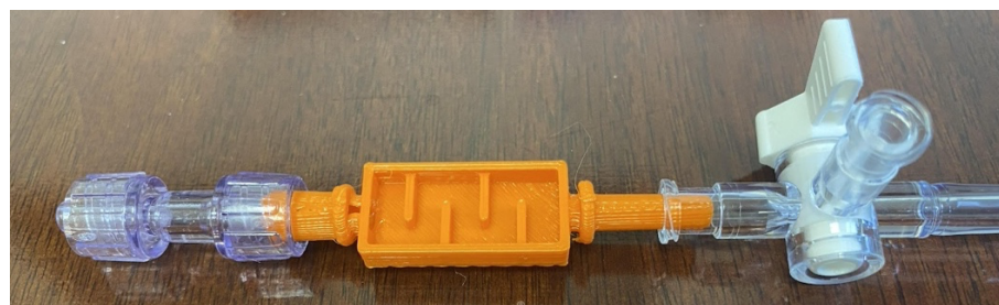
Figure 3. Dr. Thiele's initial prototype of the device. The custom 3D printed cartridge is in orange and is shown housed in the central line. UV light and power supply are not shown.
