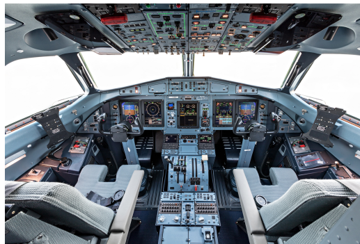
Figure 12.6: Interior of Saab 2000 Cockpit
