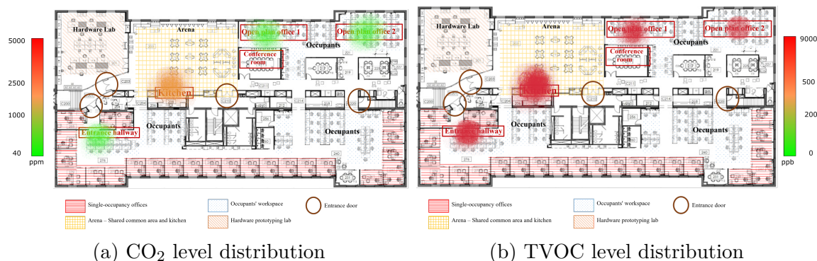
Figure 2.12: CO 2 and TVOC distribution over the lab during an event
