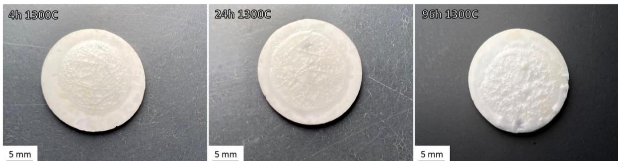
Figure 4-11. Macro images of YbPO<sub>4</sub> samples after CMAS exposure for 4, 24, and 96 hours at 1300 °C.
