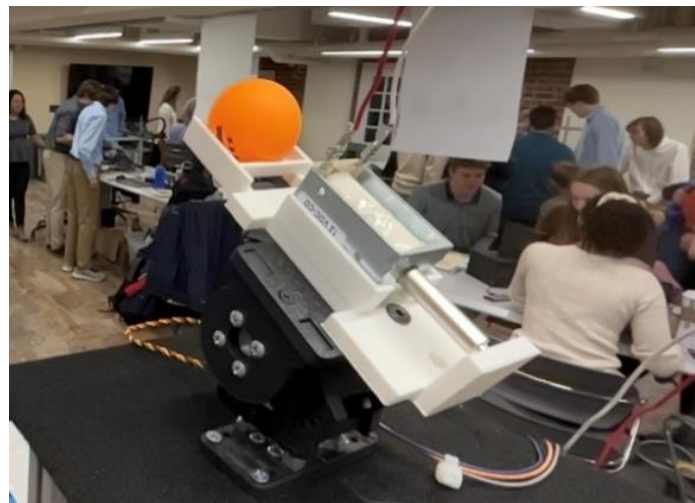
Figure 7: Solenoid Track Final Version – Mounted
