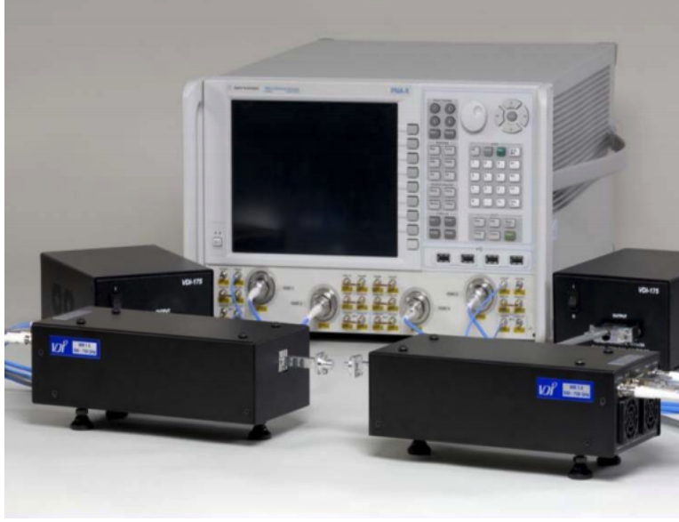
Figure 1.2: VDI frequency extension modules shown for size comparison to a typical VNA.
