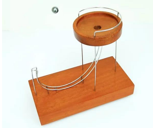
Figure 1: Pseudo-perpetual motion machine. The steel ball rolls down the ramp, then is launched off the end back to the top so that it can roll down the ramp again. As true perpetual motion is impossible, a battery-operated electromagnet is hidden in the base to accelerate the ball down the ramp. The technical project will feature multiple balls that roll down various ramps and pathways, and eventually end up back at the top to repeat the cycle. (The Awesomer, 2021).
