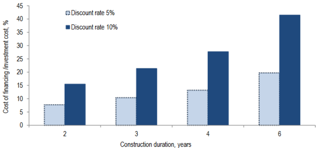
Figure 4: Cost of financing as a function of construction duration and interest rate with a uniform financing schedule (NEA, 2011).
