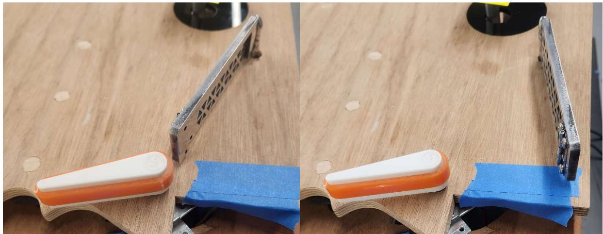
Fig. 2.5.2. Diverter gate in closed and open position
