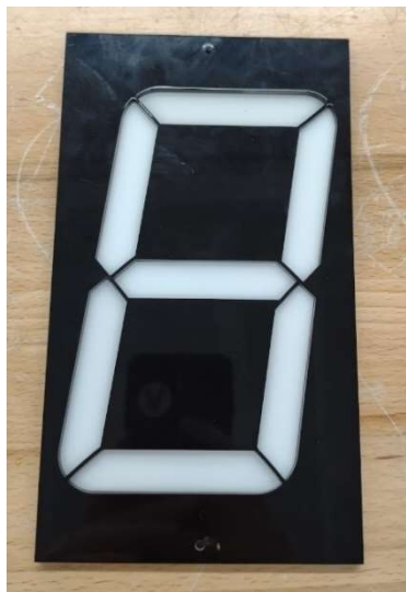
Fig. 2.10.1. Single acrylic digit prototype
