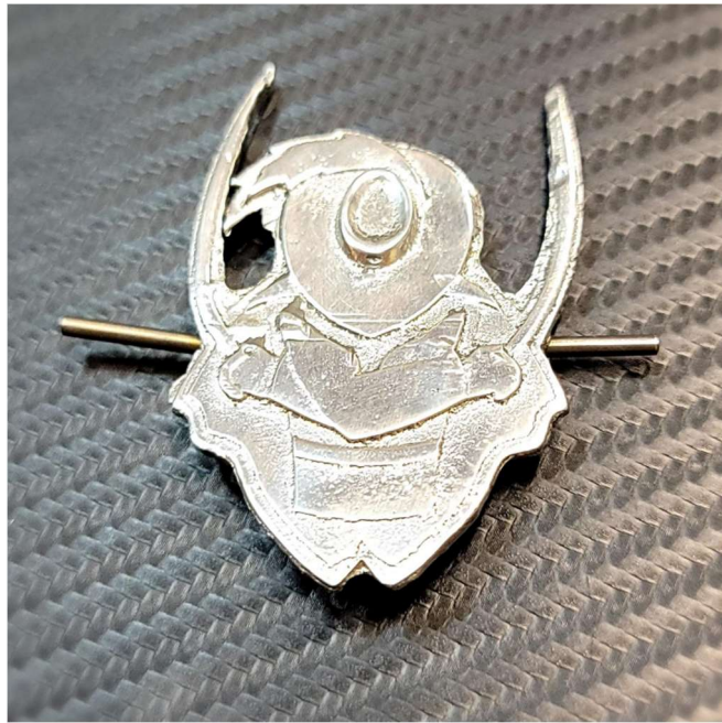
Fig. 2.8.2. First cast of Cavman spinner
