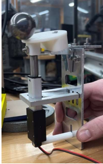
Fig. 2.6.5. Testing of the final trapdoor assembly
