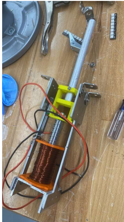
Fig. 2.3.6. Second iteration of pop bumper (pre-mounting)
