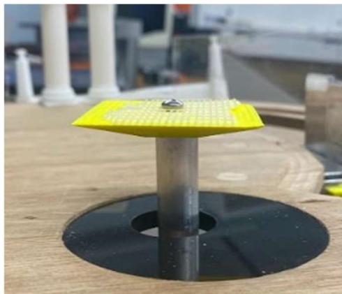
Fig. 2.3.8. Second iteration of the pop bumper mounted (above playfield view)
