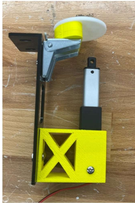
Fig. 2.6.3. First prototype of the vertical trapdoor design
