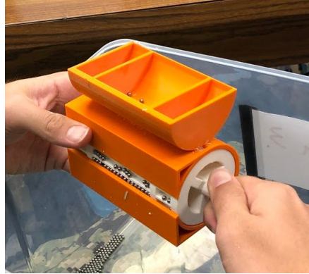
Figure 13: Spinning a preliminary model of the reservoir-drum assembly
