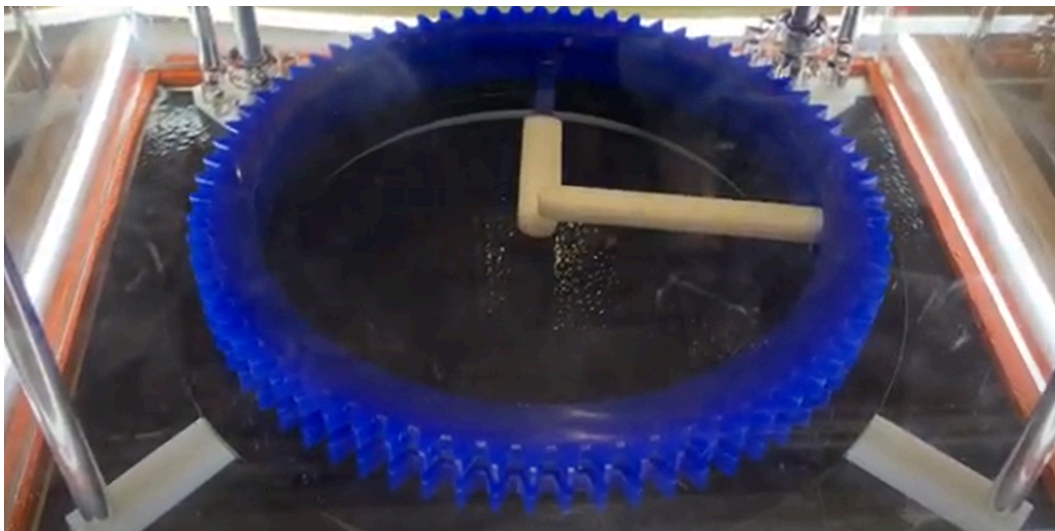
Fig. 22: An image of the final prototype with the white acrylic hands extending from the blue acrylic ring gears (created by authors).
