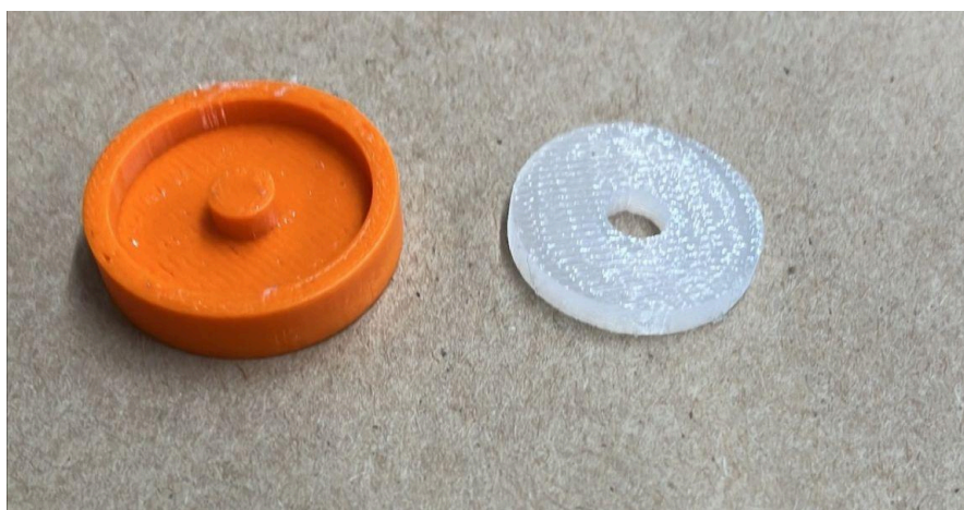
Fig. 28: Image of silicone seal ring with 3D printed mold
