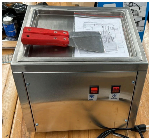
Fig. 9: The VEVOR brand ice cream machine selected for the cold plate element of the cloud chamber (created by authors).
