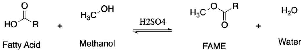
Figure 3.7-01: Esterification of free fatty acids into FAME.
