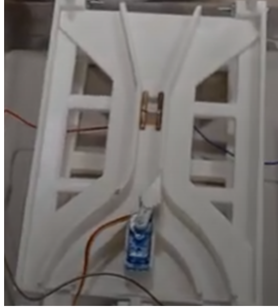
Figure 2: Conductivity Sorter Prototype for 1/2" Bearings
