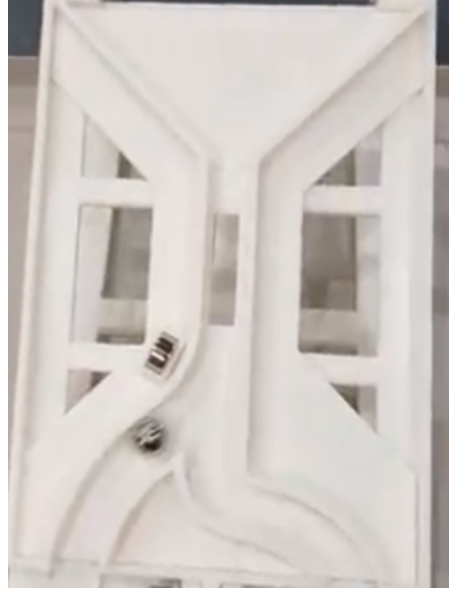
Figure 3: Magnetic Sorter Prototype for ½” Balls
