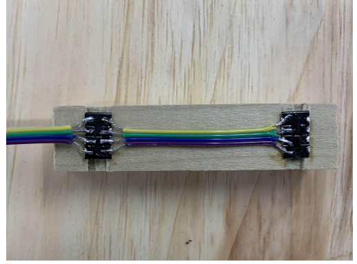
Fig. 14. Manufacturing tool to ensure consistent distances between LEDs.
