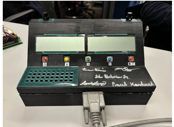
Fig. 22. Final version of the clock box. The top two buttons correspond to each of the players' turn swap, the while the others correspond to clock, hint, undo, pause, and restart, respectively.
