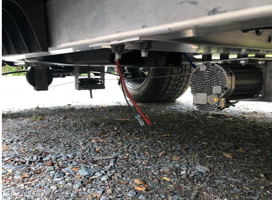
Figure 10: Installed Clearpath MC Brake Motor. (Patrick Dunnington, 2023)
