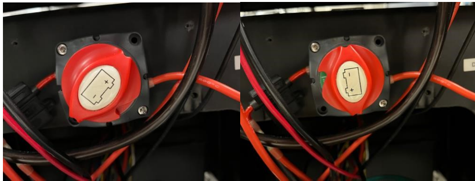
Figure A1: Switch on the back of the cart being turned on.
