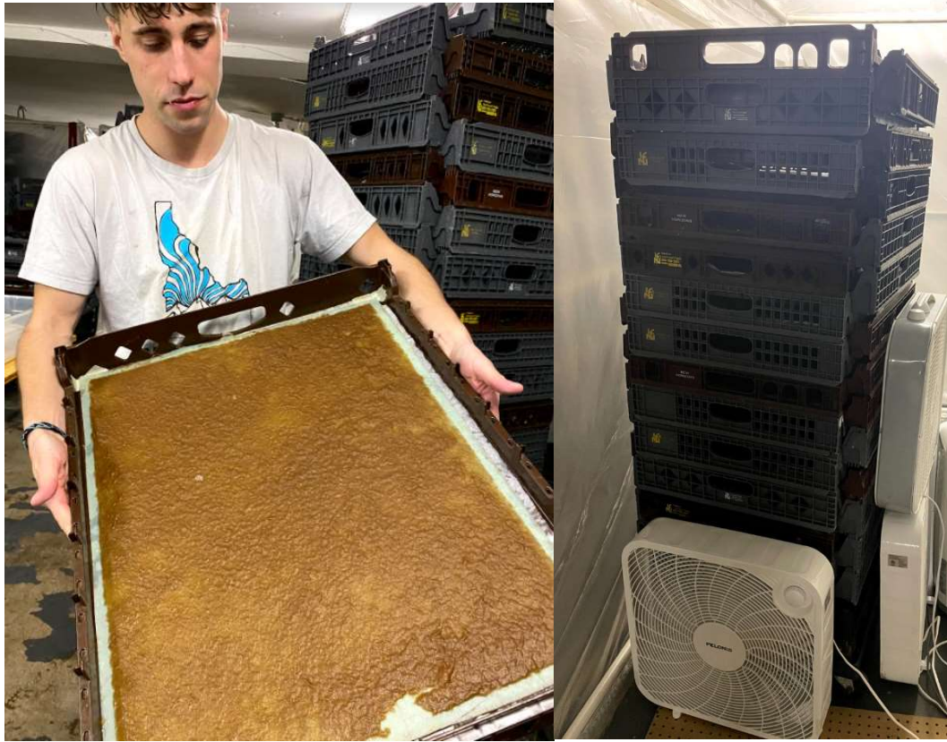
Figure 12: Sheets formed on fourdrinier fabric were removed from the SFCs and arranged in a highly ventilated stack for proper drying.
