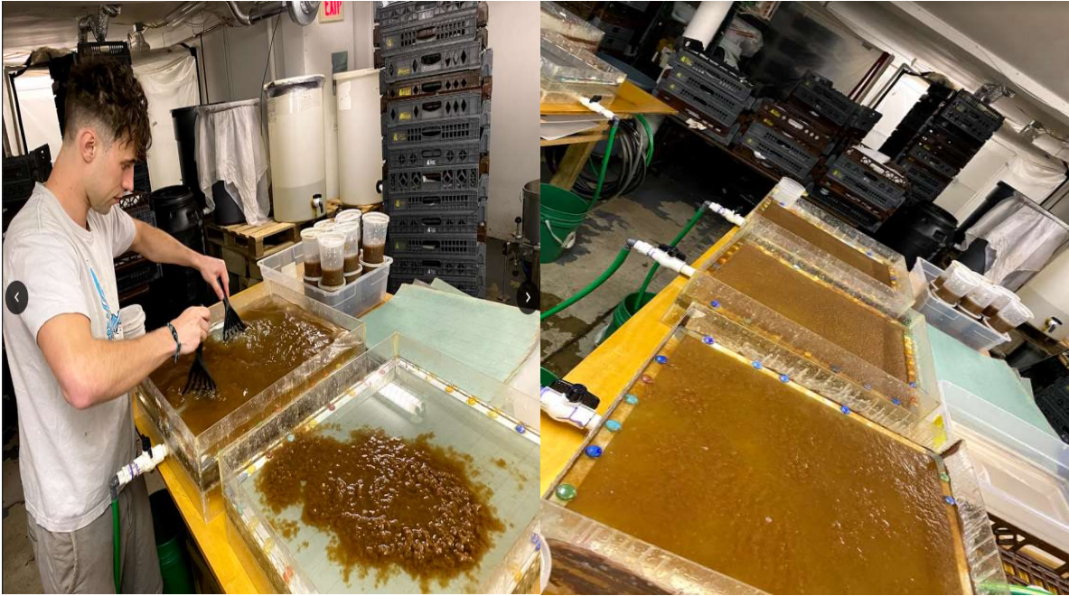
Figure 11: Pre-drainage A. homogenization of the various grades of Kraft, OCC and BNC fiber Post-drainage B. sheets formed via the drainage and filtration of the homogenized water/fiber bath.
