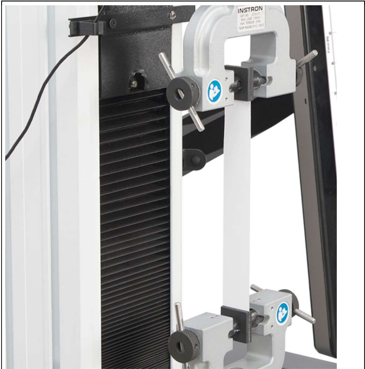
Figure 14: Displays an Instron used for paper sample tensile and strength testing. (Instron, 2020)
