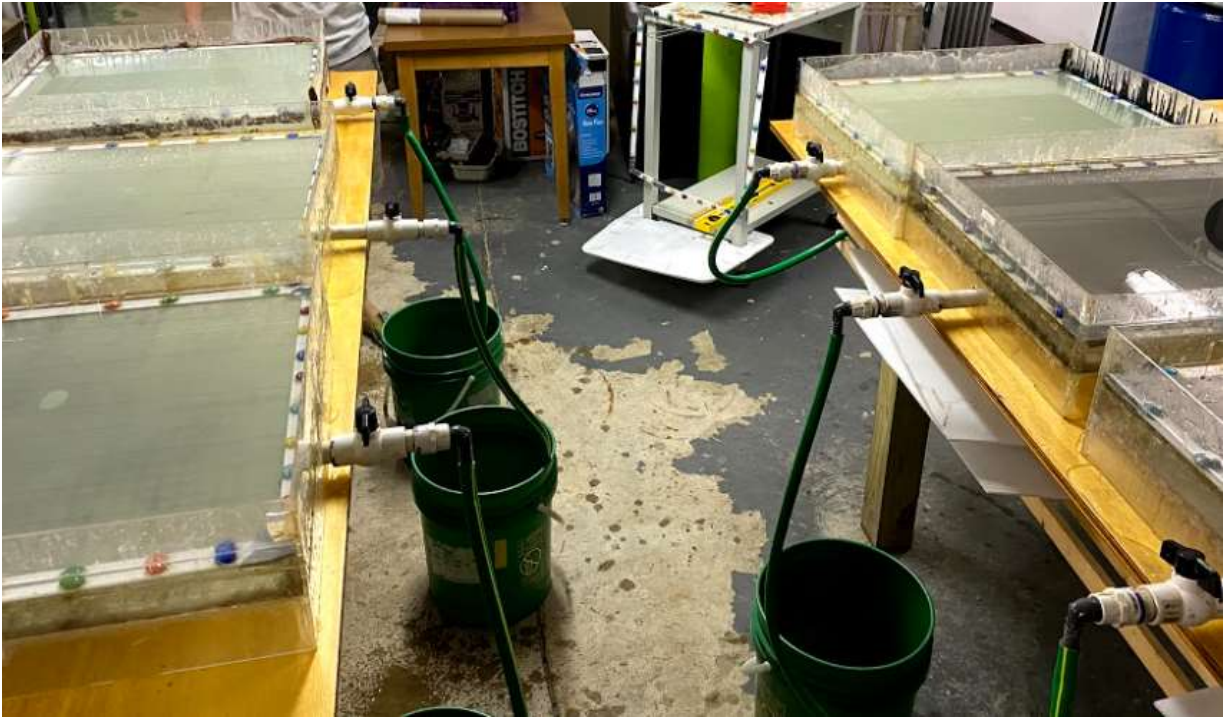
Figure 10: 6 SFCs and recyclable drainage systems set up in parallel pre and post staging with water and border-weighted fourdrinier catching/drying stage.
