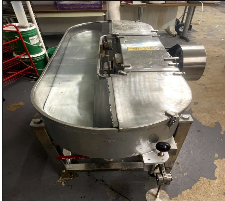
Figure 8: Shows the Hollander beater. The right side houses the maceration mechanism operated by a belt driven turbine. Bottom right of the picture shows the lever that controls the gauge length. The left half of the Hollander beater is open face allowing for pulp consistency to be monitored while pulping is in progress.
