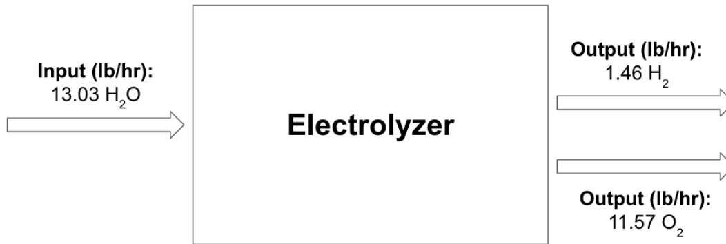
Figure 3.3.2. Material Balance for the Electrolyzer
