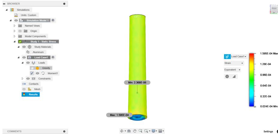
Figure 18: Finite Element Analysis of the Strain for a Solid Load Cell Structure
