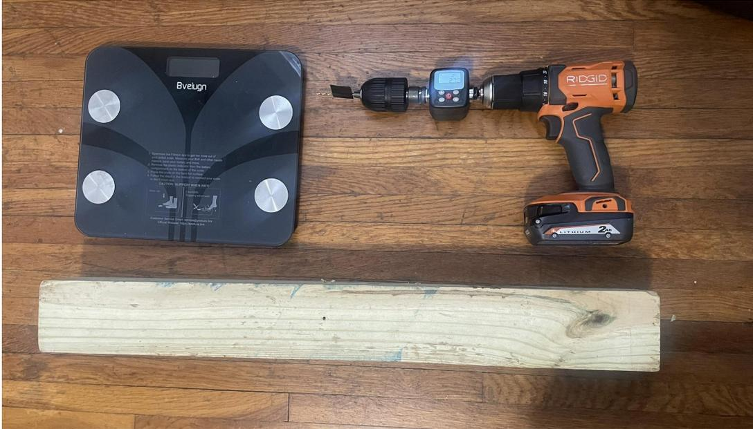
Figure 16: Experimental Setup Consisting of Bathroom Scale (Top Left), RIDGID Handheld Cordless Drill with Precision Torque Wrench Adapter and Square Drive to Jacobs Chuck Adapter (Top Right), and 4x4 Yellow Pine Sample
