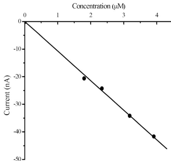
**Figure 4.1 Calibration of oxygen.** The oxygen concentration was calibrated using nitrogen- and air-saturated PBS buffer with volume ratio of 1:0, 2:1, 5:1, 10:1, and 15:1. Nitrogen-saturated PBS buffer without oxygen was used as running buffer. The linear equation is  $y = -0.34x$  ( $R^2 = 0.99$ ). This graph allows calculation of oxygen concentration.
