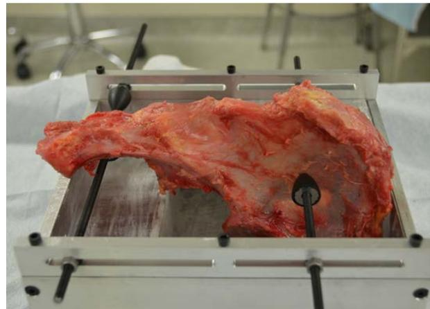
**5.1.2-1 – Potting cup; plungers helped hold the pelvic wing in place while pouring the resin to ensure that the wing did not move as it was secured into its desired orientation.**
