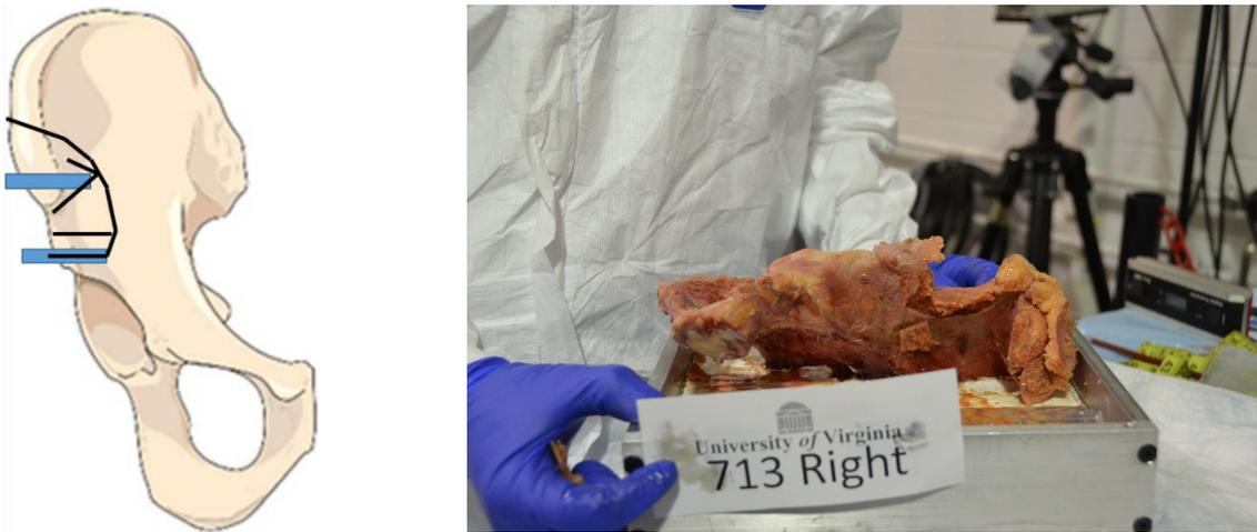
**5.2.3.1-1 Fracture Diagram of Test 713R ("Snapping" Fracture). Blue boxes indicate the top and bottom edge of the seatbelt webbing**
