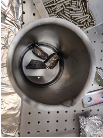
Figure B.2: Lithium. (a) 95% isotope of {}^6\text{Li} chunk. (b) Image after baking {}^6\text{Li} chunk in the oven section. To eliminate the mineral oil layer on the surface, a Pentane rinse is performed, followed by baking to remove any oxidized layers. Note that Acetone cannot be used due to its potential to oxidize {}^6\text{Li} . To minimize oxidation when in contact with air, we flush argon during the process.
