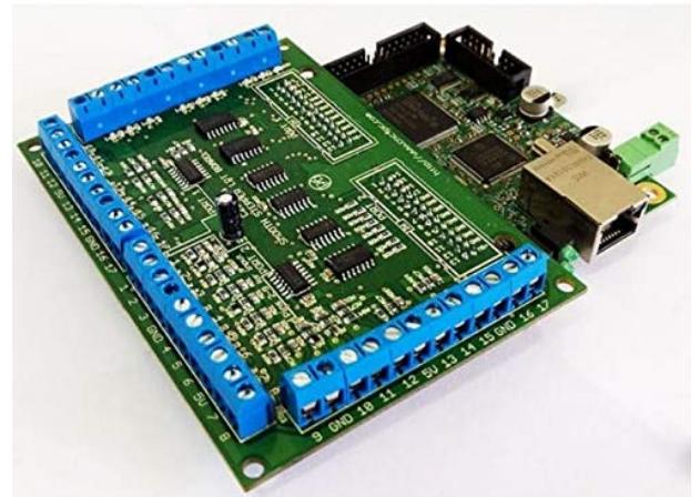
Figure 1: ESS Motion Control Board with Terminals for Mach3 & Mach4 Software. Image taken from Amazon.com.
