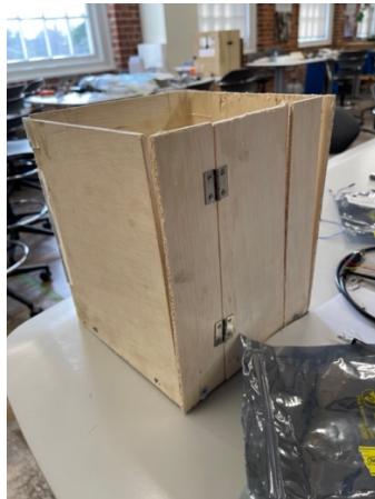
Figure 1: Prototype of the Wooden Enclosure of the “Tap Box” that Holds all Electrical Components Inside
