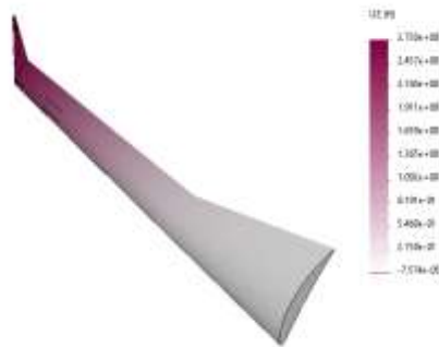
Fig. 6-19. Wing flex deformation for full-payload takeoff
