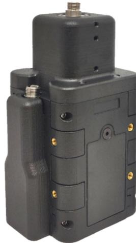
FIGURE 4.5: **PICAS system.** The push beam couples in to the central fiber jack in the rear, the 2D MOT beams couple in to the other two fiber inputs (one pictured). This system contains permanent magnets within and optics used to produce the 2D MOT beam. When mounted, it fully encloses the 2D MOT cell.
