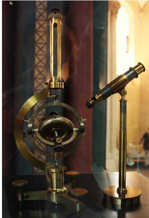
(B) Replica of spinning gyroscope designed by **Leon Foucault**. A spinning gyroscope based on a Serson speculum gyroscope. This type of gyroscope was used in first detecting the rotation of the earth. [19]
