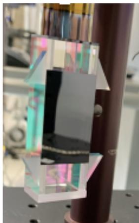
FIGURE 4.6: A photograph of the 3D MOT vacuum cell. The cell by itself with the Bragg mirrors attached and silicon membrane featured prominently.
