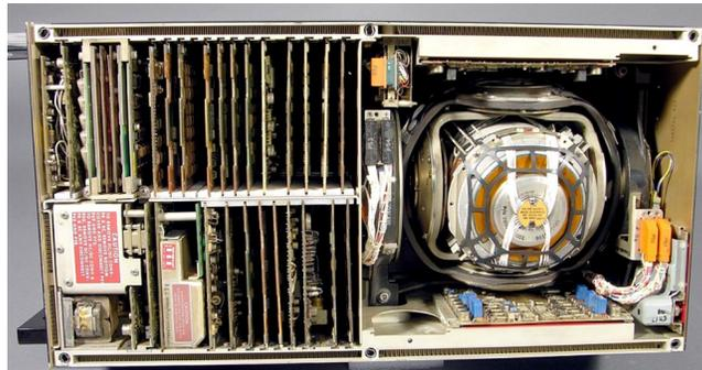
FIGURE 1.1: **Transatlantic flight display INS.** Non-operational prototype made for display purposes by the Delco Division of General Motors. The Delco Carousel dimensions were  $25.4 \times 54.6 \times 20.3$  cm. [5]
