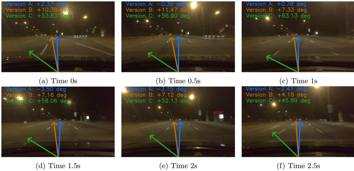
Figure 3.21: A sequence of camera images that produced a steering difference of more than 45 degrees, for at least 38 frames (approximately 2.5 seconds), that were in-ODD, identified by our approach.
