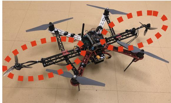
Figure 4.7: Two-arm haptic suit prototype (marked using dashed lines) mounted on a DJI Flamewheel F450 drone [85].
