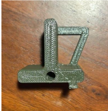
Fig. 23. Flipper with new preventative arm and tab (bottom)
