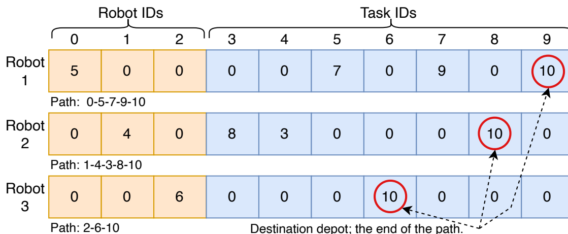
Figure 5.3: Graphical representation of chromosome encoding.
