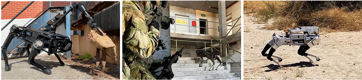
Figure 7. VISION 60 Q-UGV performing various defense/homeland scouting tasks with different attachments on its back (7a Left, 7b Middle, and 7c Right) (Ghost Robotics, n.d.-a).
