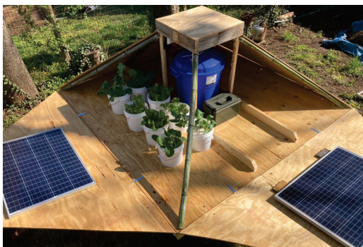
Figure 4. Prototype floating platform, partially folded.
