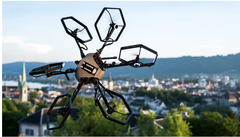
Figure 1.5: The Voliro hexacopter’s tilting rotors let it hover and fly in any orientation. (copyright: Voliro [81])
