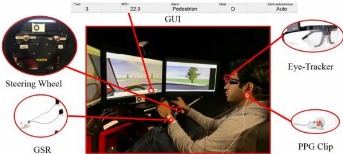
Figure 2: Each participant was seated in the driving simulator and outfitted with a series of physiological monitoring devices such as an eye-tracker, galvanic skin response (GSR) sensor to track stress responses on the skin, and a photoplethysmography (PPG) sensor to track heart rate. Additionally, during each test the participant reported their trust electronically using the graphical user interface (GUI) shown above, while receiving information about the vehicle's status through that same GUI. Taken from the published paper from the research project (Sheng, et al. 2019)
