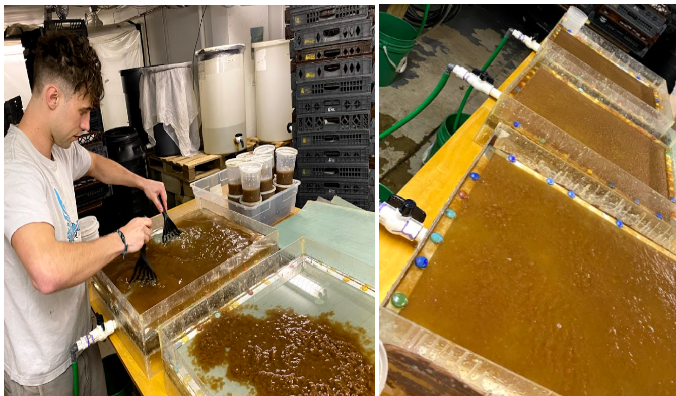
Figure 11: Pre-drainage A. homogenization of the various grades of Kraft, OCC and BNC fiber Post-drainage B. sheets formed via the drainage and filtration of the homogenized water/fiber bath.
