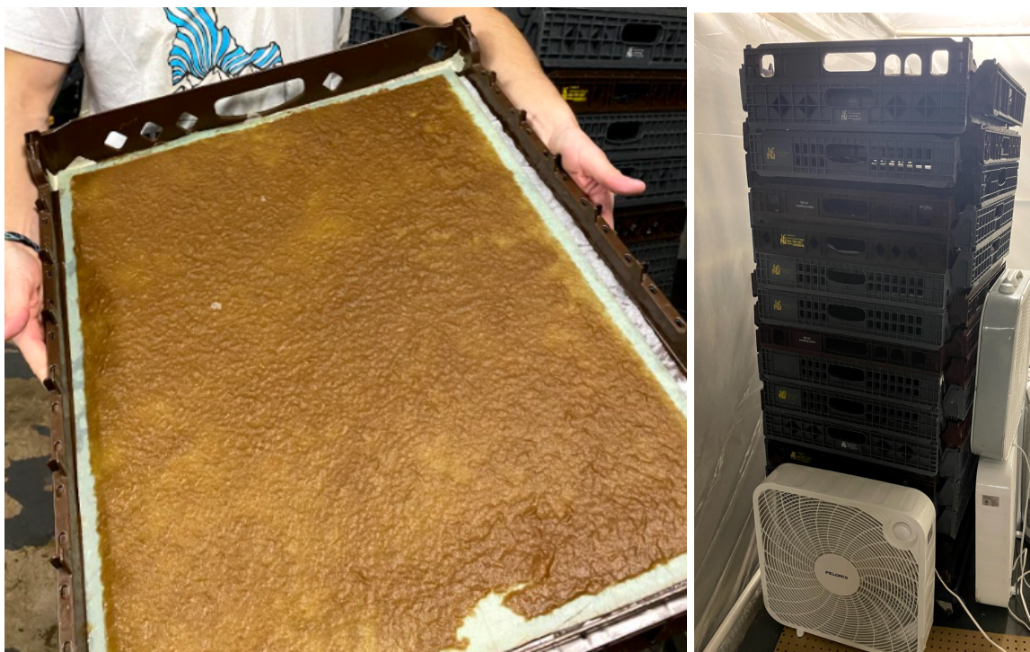
Figure 12: Sheets formed on fourdrinier fabric were removed from the SFCs and arranged in a highly ventilated stack for proper drying.
