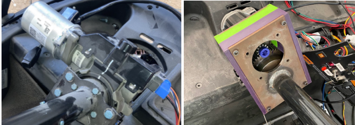
Figure 3 : Nexteer electric power steering system (left); Teknic ClearPath Servo Motor with gears housed in an enclosure (right).
