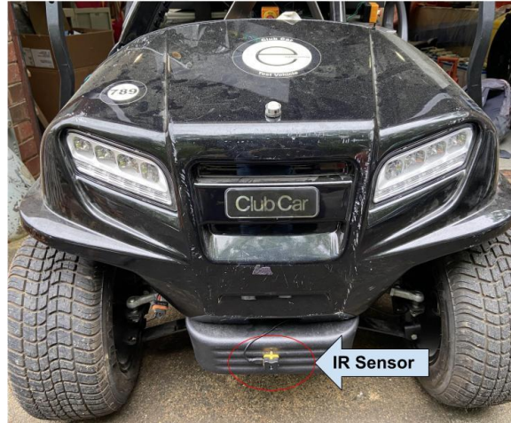
Figure 19: Location of IR sensor at the front of the follower cart.
