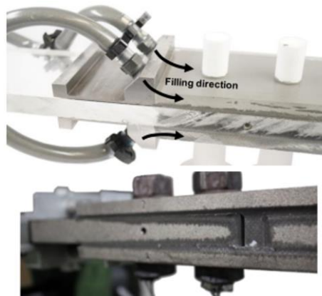
Figure 3. Images of steel connection injected with epoxy (Makevičius et al., 2021)
