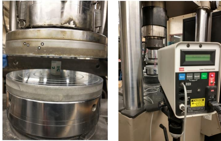
Figure 26. MTS compression test setup and laser setup.
