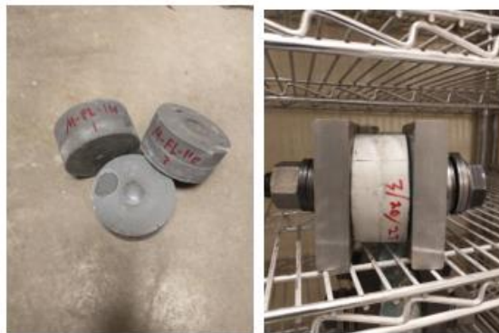
Figure 29. Compression creep assembled rig with cured adhesive specimen
