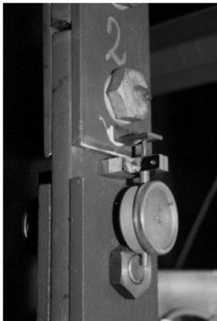
Figure 22. Tensile creep test for injection bolted connection (Gresnigt, 2000)
