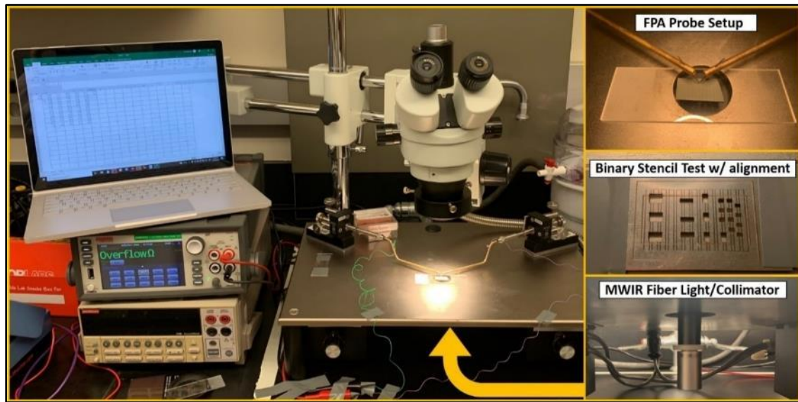
Figure 78: Modified probe station for operational testing of the FPA prototype by backside projected illumination.
