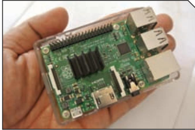
Figure 4: A Raspberry Pi (Stehmeyer, 2016, 2)
