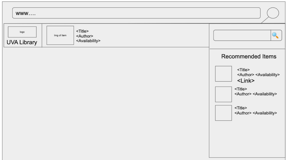
Figure 1: A wireframe diagram outlining the general interface seen by UVA Library Chrome extension users searching for books (Created by Author).
