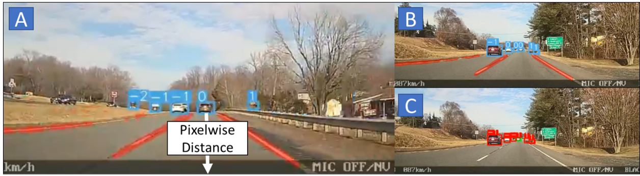
Figure 5.6: The methodology to calculate the pixelwise distance from the lead vehicle. (A) detection the lead vehicle using a combination of lane tracking and object detection. Enhancing the high number of false positives in detection as the lead vehicle (B) through post-processing (C)
