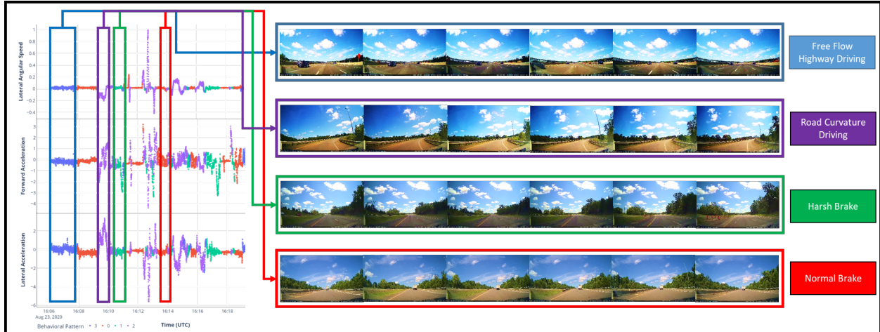
Figure 4.10: Samples of the detected driving patterns. Patterns 0 and 1 are associated with normal and harsh braking behavior, while pattern 2 is associated to curve driving behavior, and pattern 3 is related to highway free flow driving behavior.
