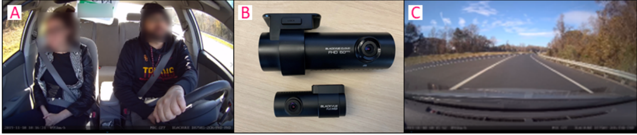
Figure 3.2: sample view of the in-cabin camera (A), BlackVue dash camera (B), sample view of the outside cabin dash camera (C) ©2021 IEEE
