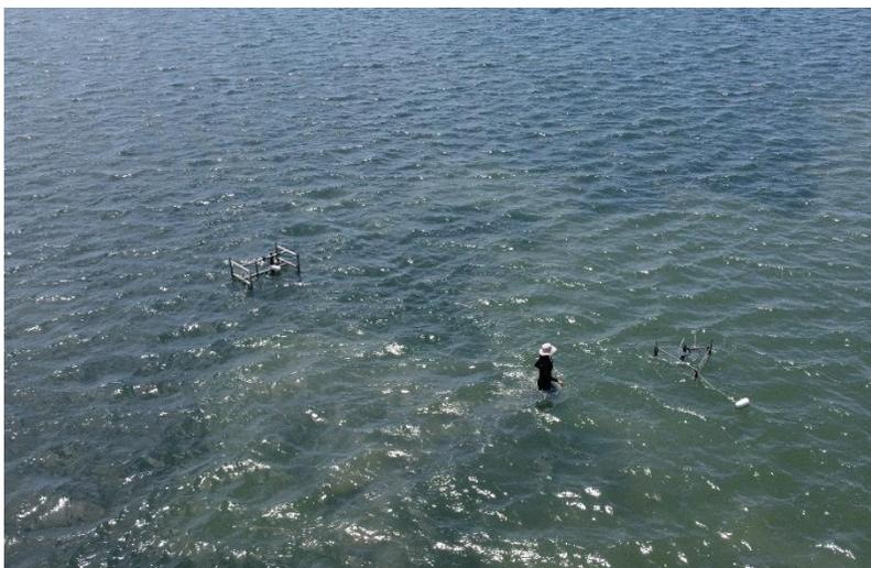
**Photo 2.5.** Drone photo taken by Spencer Tassone showing two Vector instrument frames deployed across the meadow's natural edge of vegetation at Site 2 in summer 2022.
