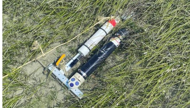
**Photo 2.1.** Instrument frame with Aquadopp (black) and RBRduo<sup>3</sup> (white) in vegetation.
