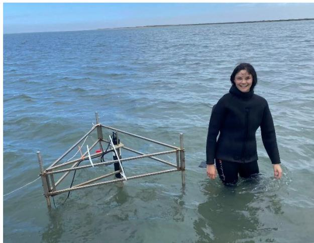
**Photo 2.2.** (Left) Vetrino instrument (black) secured to instrument frame recording instantaneous velocity data over seagrass vegetation. **Photo 2.3.** (Right) Vector instrument (black) secured to weighted instrument frame over seagrass vegetation.
