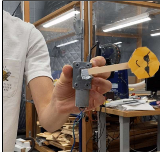
Figure 13: Worm gear motor with prototype sun arm attached
