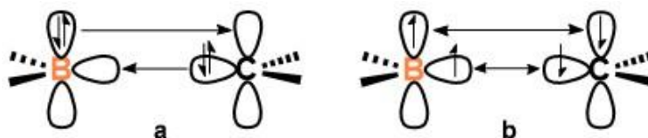
Figure 4.5. Bonding models considered for EDA, a) Singlet fragment donor-acceptor model, b) Triplet fragment electron-sharing model.
