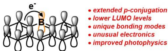
Figure 1.7. Schematic depicting the empty p_z -orbital of boron accepting electrons.
