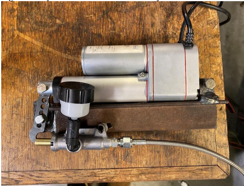
Figure IV. Linear actuator and master cylinder
