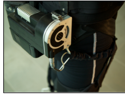
Fig 3. Bowden cable mechanism [10]
