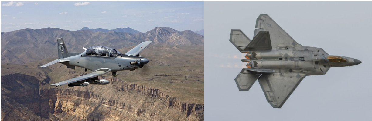
Figure 1: AT-6 Wolverine (Left) vs the F-22 Raptor (Right), notice the low wing design and the numerous missile and bombs connected to the hardpoints for ground strikes for the AT-6, while the F-22 has a sleek design meant to move fast and utilizes internal bomb bays to strike the enemy. (AT-6 Wolverine, n.d., Ritsick,2020)
