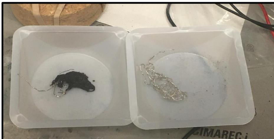
**Figure B10.** Pt mesh coated from viscous DAFc<sup>+</sup> solution after performing bulk electrolysis on 100 mM DAFc (sample on left). A clean Pt mesh on the right is displayed for comparison.
